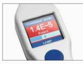
The search results are presented on the hand probe's screen, simplifying leak detection.
