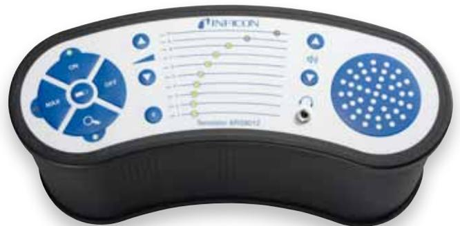
To be able to detect both minor and major leaks Sensistor XRS9012 features a sensitivity adjuster to instantly adapt to any detection condition. The electronic sensor mounted in the probe tip responds instantaneously to the tracer gas, and additionally the instrument has a very short recovery time to enable new measurements to be performed immediately.
