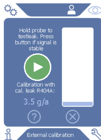
Fig. 14: Display when calibrating externally
