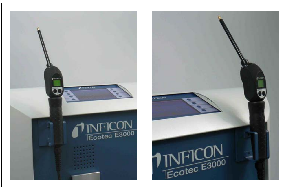
Fig. 1-7 Usage of sniffer line holder
