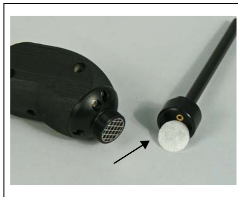
Abb. 7-11 Removed filter pad
