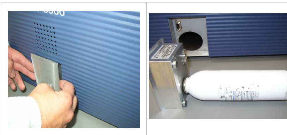
Fig. 7-17 Removing the PRO-Check reference leak from the main unit
