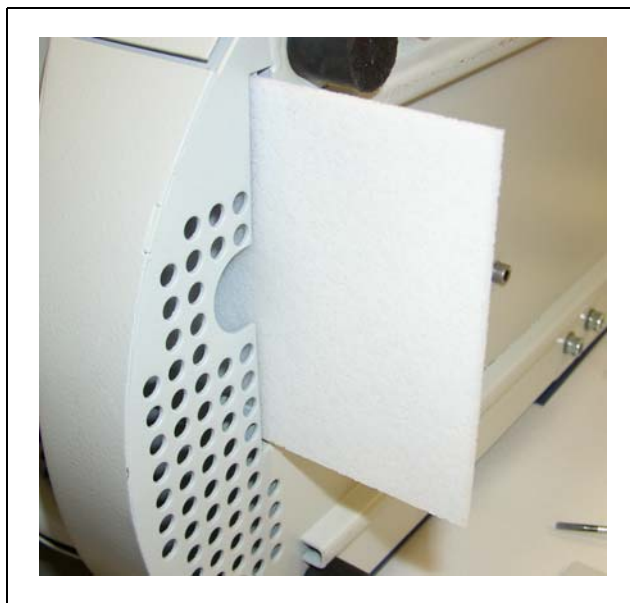
Fig. 7-3 Inserting the air filter
