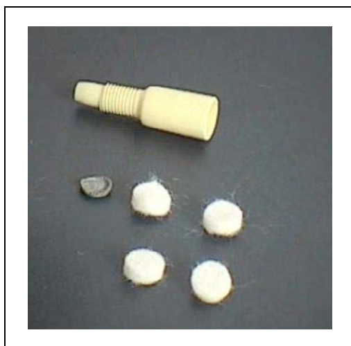
Fig. 7-7 old and new felt filter
