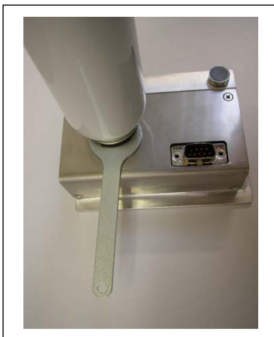
Fig. 7-19 Installing the gas reservoir
