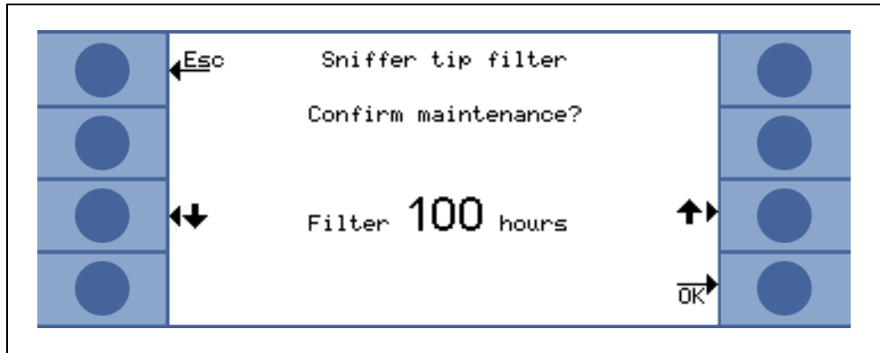
Fig. 4-22 Setting the maintenance interval for the sniffer tip filter and confirming its replacement
