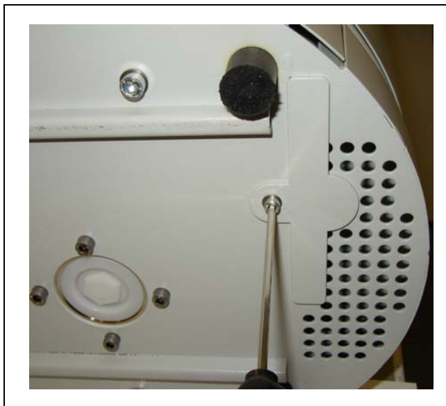
Fig. 7-1 Fastener for the air filter on the bottom of the leak detector
