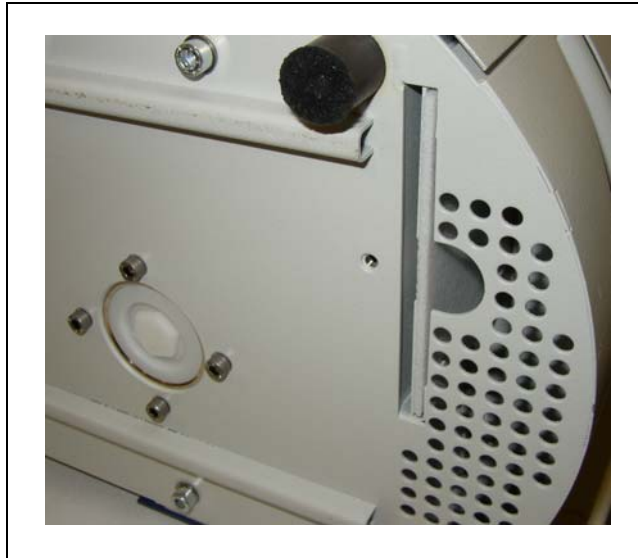
Fig. 7-2 Dismounting of the air filter
