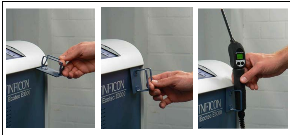
Fig. 1-8 Installation of sniffer line holder
