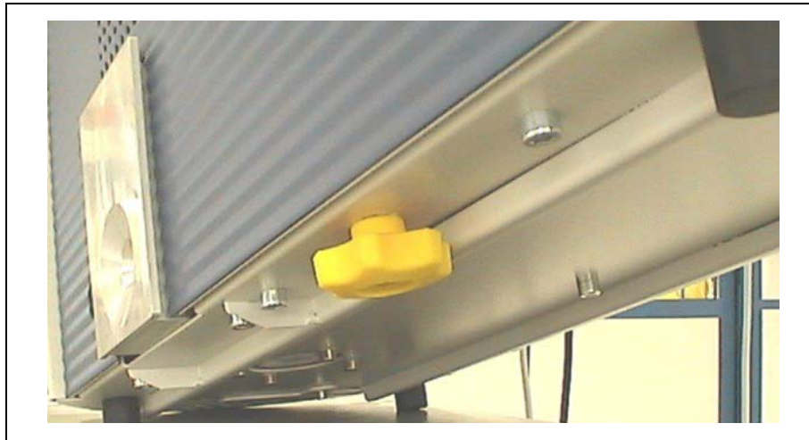
Fig. 1-3 Removing the transportation lock before starting
