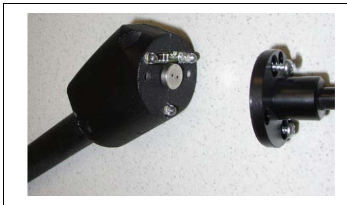
Fig. 7-8 Taking off the sniffer tip
