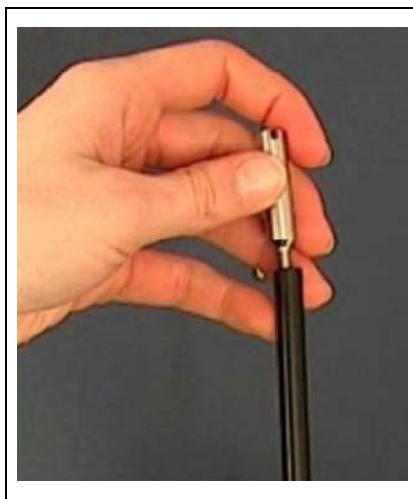
Fig. 1-4 Installing water protection tip
