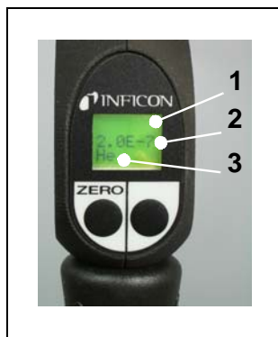
Fig. 3-5 Sniffer display in standard operation mode
