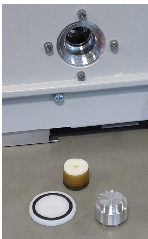
Fig. 49: Opened operating fluid reservoir
