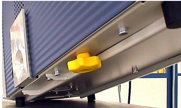
Fig. 5: Unscrew the yellow transport restraint before the start-up
