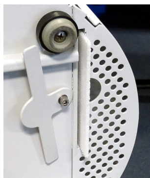
Fig. 47: Air filter in the air filter duct
