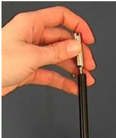
Fig. 8: Tightening the water conservation sniffer probe
