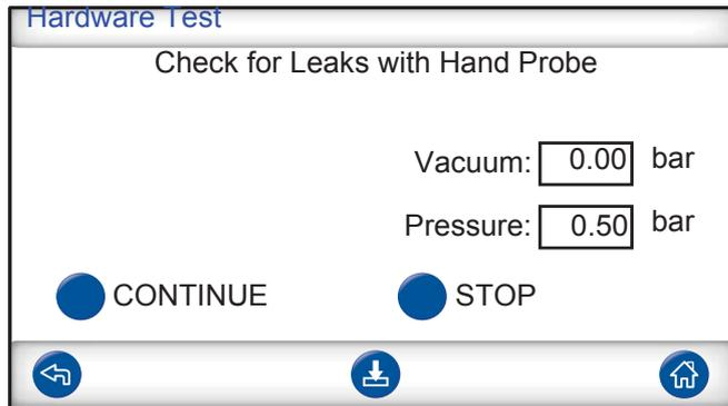
The ILS500 is now prepared for a manual test for external leakage. Use the hand probe to check for leakage
