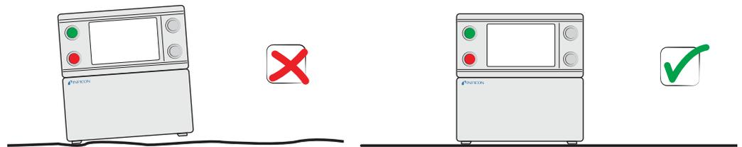
Place the ILS500 on a flat surface, as close as possible to the test fixture and ventilation system.
