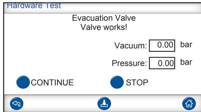
This step tests that evacuation valve opens to release tracer gas to exhaust. Same test as previously but under pressure instead of vacuum.
