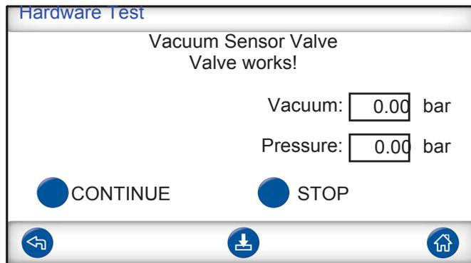
This checks that the valve shuts to protect vacuum sensor before filling.
