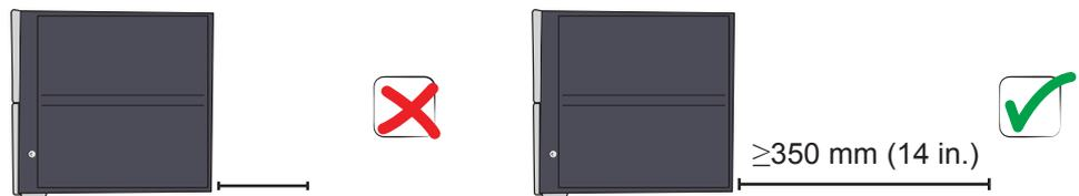
Ensure that there is at least 350 mm (14 in.) of free space behind the ILS500 to enable removal of service hatches, connection of supplies, test fixture etc.
