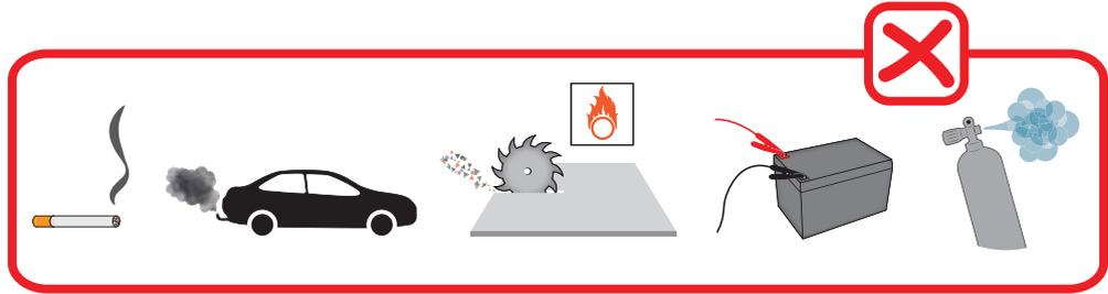
Avoid to place the ILS500 close to hydrogen sources such as cigarette smoke, combustion engines, aluminum machining, lead battery charging stations and compressed air systems.
