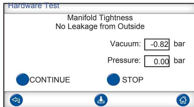
The overall tightness of the manifold is tested using the vacuum raise method.
