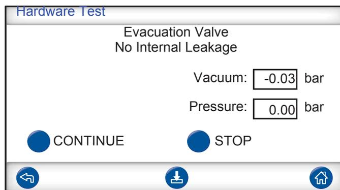
Evacuation valve is checked for internal leakage.
