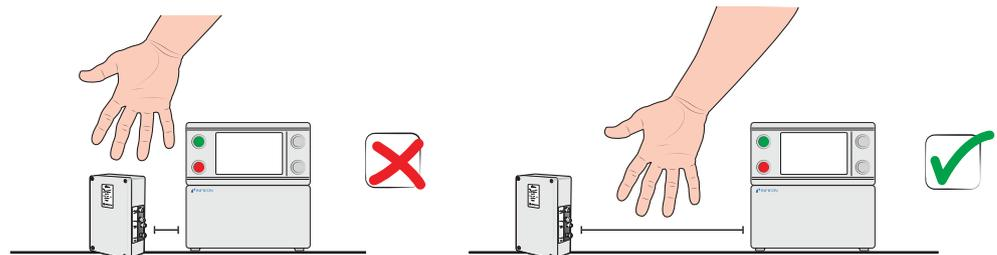
Some free space must be provided around the ILS500 to enable maintenance and service access.
