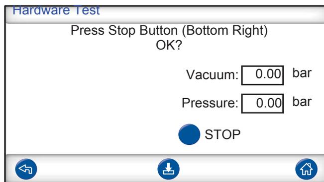
This is a “manual” test. The test continues when the correct button is pressed. The test checks the activated START and STOP buttons only. Use INPUT menu under Service menu to check buttons that are turned off.
