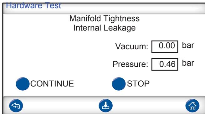
The overall tightness of the manifold is tested using the pressure decay method. This is a complement to the gas test, revealing leakage out, through the exhaust etc.
