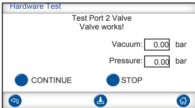
**Notice** This test will fail if both test ports are connected to a test object. Proceed and then repeat the entire hardware test sequence with both ports plugged to perform this test step.
