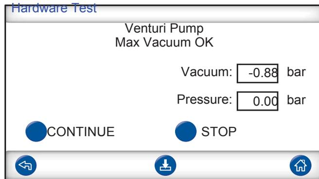
Checking max vacuum of Venturi pump.
