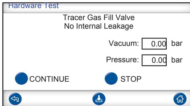
The step tests the gas fill valve for internal leakage by registering pressure rise behind the valve.
