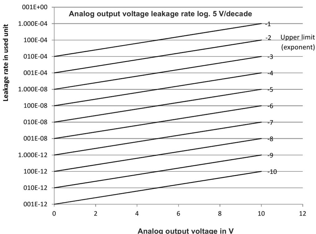
Fig. 9: Analog output voltage leak rate log. 5 V / decade
