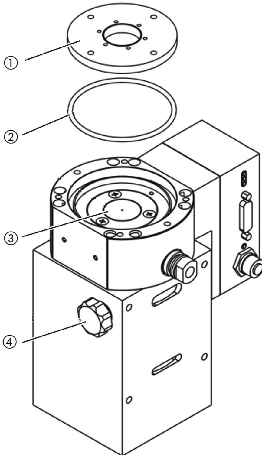
Fig. 14: Turbo molecular pump SplitFlow 80
