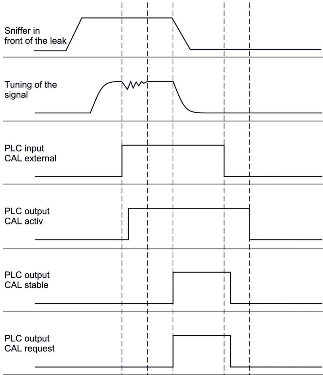
Fig. 6: External calibration with IO1000 using the example of sniffer line SL3000XL, description of PLC inputs and outputs: "Assigning inputs and outputs [▶ 55]"
