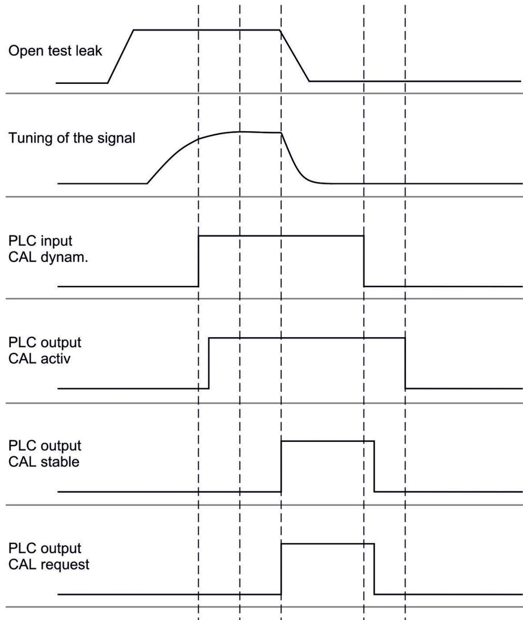
Fig. 7: Fig. 7 External dynamic calibration with IO1000 using the example of sniffer line SL3000XL, description of PLC inputs and outputs: "Assigning inputs and outputs [▶ 55]"
