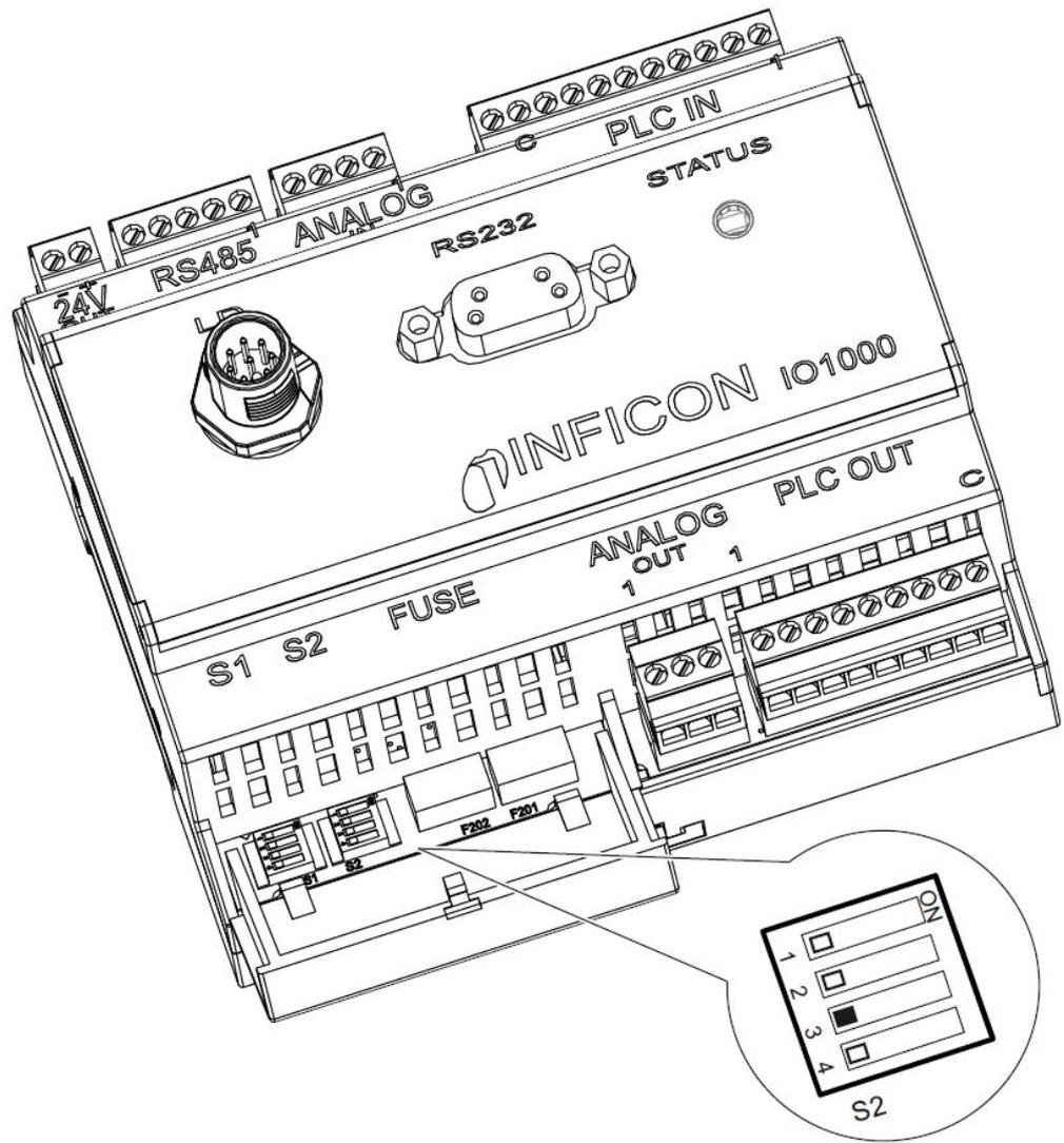
Fig. 13: DIP switch on the I/O module
