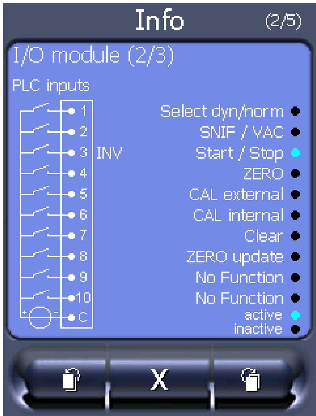
Fig. 11: I/O module (2): Visualized information to the digital inputs
