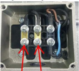
The motor must be connected according to the electrical codes through a fused switch in order to protect the motor against electrical or mechanical overload conditions. The overload of the motor starter must be set at a level equal to the full load motor current listed on the motor nameplate.
