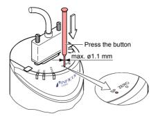
**2** For changing the threshold value, push the <ZERO> button and keep it depressed. The threshold keeps changing from the current value (ramp) until the button is released or until the limit of the setting range is reached.
