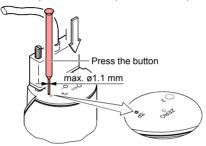
For changing the threshold value, push the <ZERO> button and keep it depressed. The threshold keeps changing from the current value (ramp) until the button is released or until the limit of the setting range is reached.
