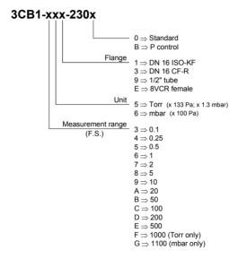
The part number (PN) can be taken from the product nameplate. If not indicated otherwise in the legends, the illustrations in this document correspond to gauges with the DN 16 ISO-KF vacuum connection. They apply to other vacuum connections by analogy. We reserve the right to make technical changes without prior notice. All dimensions in mm.
