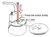
After zero adjustment the gauge automatically returns to measurement mode
