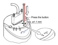
For changing the threshold value, push the <ZERO> button and keep it depressed. The threshold keeps changing from the current value (ramp) until the button is released or until the limit of the setting range is reached.
