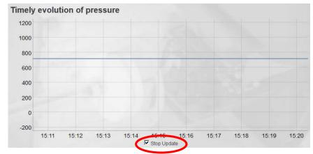
Checking the <Stop Update> box stops the data refresh. Any zoom will remain in effect. Unchecking the box will resume normal refresh. The graph is automatically updated to display all data.
