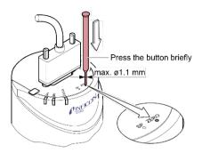
... apply supply voltage to Remote Zero at pin 10 (pulse  $\rightarrow$   $\bigcirc$  9).
