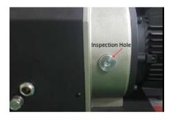
Inspection hole with G1" plug: Check the coupling and its insert, and fan through this hole regularly. (An endoscope or WireCam can be used with Smart Phone software)
