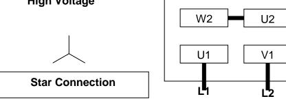
The motor must be connected according to the electrical codes through a fused switch in order to protect the motor against electrical or mechanical overload conditions. The overload of the motor starter must be set at a level equal to the full load motor current listed on the motor nameplate.
