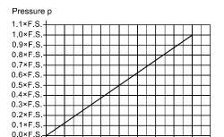
$$p = [(I_{out} - 4 \text{ mA}) / 16 \text{ mA}] \times p (F.S.)$$
