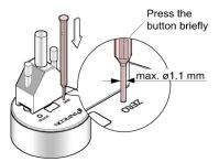
... briefly apply the supply voltage to pin 4 (Remote Zero,  $(\rightarrow \text{diagram} \ \ \ \ \ \ \ \ \ \ \ \ \ \ \ )$  16).
