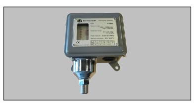
The Eurovacuum mechanical adjustable vacuum switch is specially designed to switch on/off many different kinds of vacuum pumps on the preferred vacuum level. By means of turning the button on the top of the controller it is possible to set the vacuum level on which the switch is switched off and the hysteresis (pressure difference between switching on/off) button on the side of the unit is used to set the point on which the switch is turned on again.
