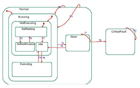
After the start, the gauge independently runs through the INIT and SELFTESTING status and eventually changes to the IDLE status (if there is no error) or to the SELFTEST\_EXCEPTION status (if there is a gauge error).
