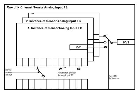
The figure below shows the basic design of the analog input function block.
