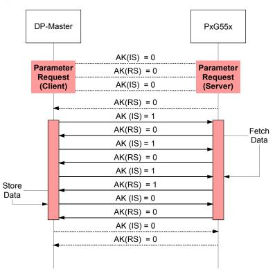
The master must mark the end of the instruction cycle by setting AK to zero. Only after that, a new instruction/response cycle may be started.
