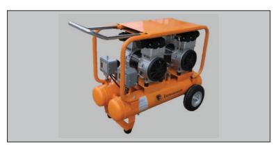
Double-level vacuum system with two 12 litre tanks, two vacuum pumps and two separate automatic vacuum level control units. The vacuum level control units can be set at vacuum levels between 100 to 1000 mbar and also the hysteresis is adjustable. This system allows the user to work at two different vacuum levels independent from the other. There is also a interlock valve on the system that connects both tanks to use the full capacity of both pumps on one vacuum level.
