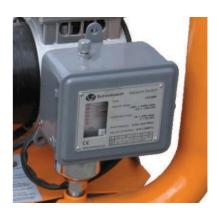
Portable vacuum system which in the transport frame integrated 2 litre tank and automatic vacuum level control unit. The vacuum level control unit can be set at vacuum levels between 100 to 1000 mbar and also the hysteresis is adjustable. This unit can hold different dry piston vacuum pumps. As the dimensions and the weight of this unit are low it is a very easy unit to take to different working locations where there is a temporary need for vacuum.
