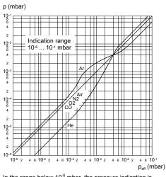
In the range below 10<sup>-5</sup> mbar, the pressure indication is linear
