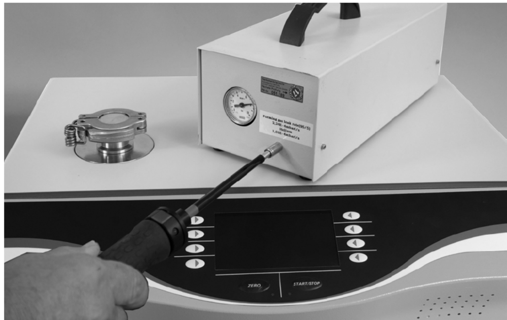
Fig. 17: Sniff test on an external calibration leak
