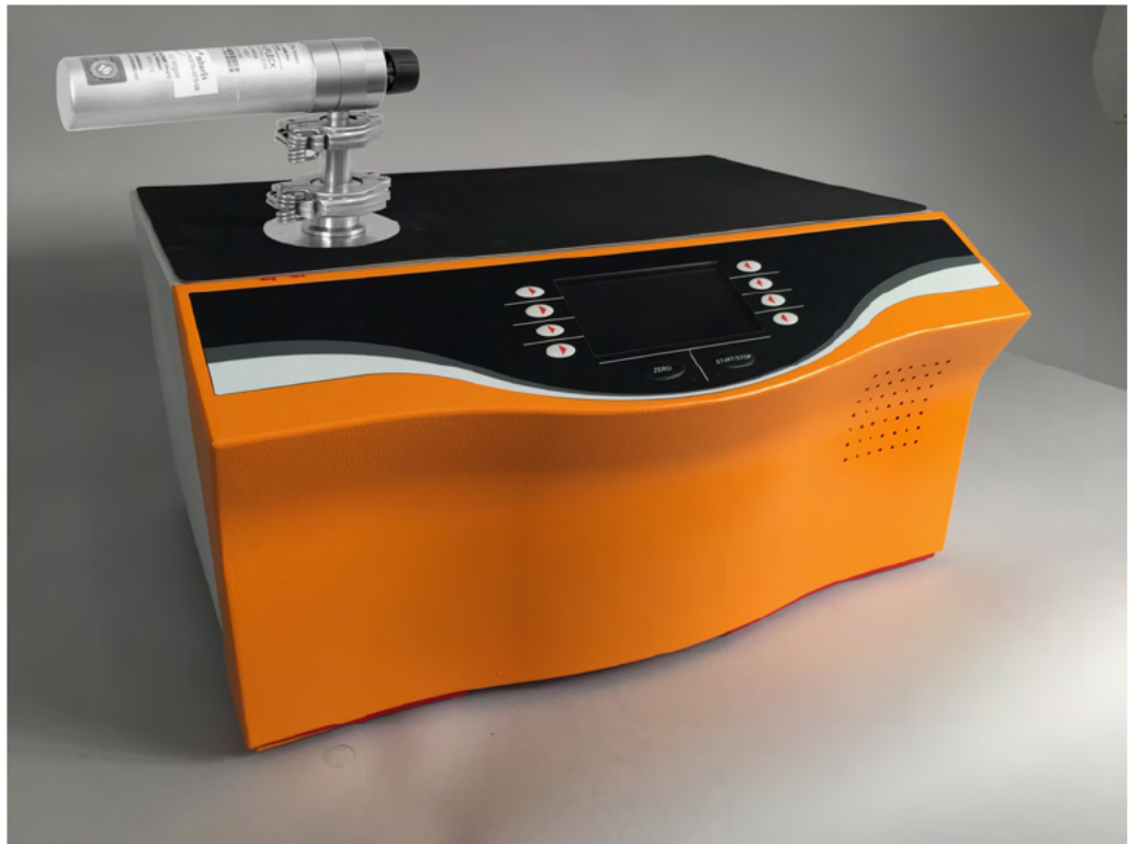
Fig. 15: Checking an external calibration leak
