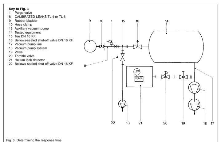
$\geq$  10<sup>-4</sup> mbar·l·s<sup>-1</sup>. As the flow rate of CALIBRATED LEAK TL 6 is between molecular and laminar flow, the correction factor can merely be assessed. Calibrated leak capillaries are manufactured by hand as single pieces and have varying lengths and diameters and hence varying flow profiles affecting the conversion factor.
