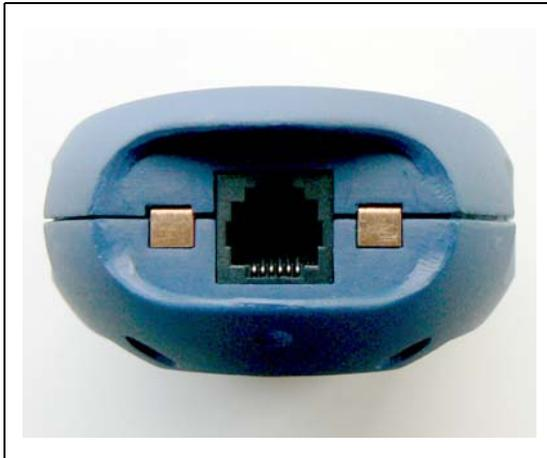
Fig. 4 RJ25 socket on the bottom of the remote control
