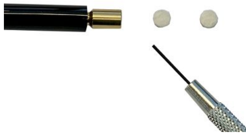
Fig. 1: Sniffer tip SL3000 with cotton filters removed
