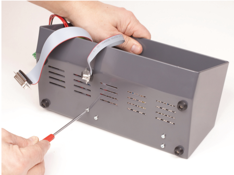
Figure E-9: Remove power supply
