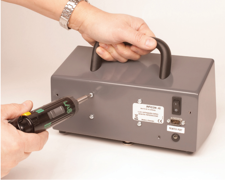
Figure E-13: Remove screws
