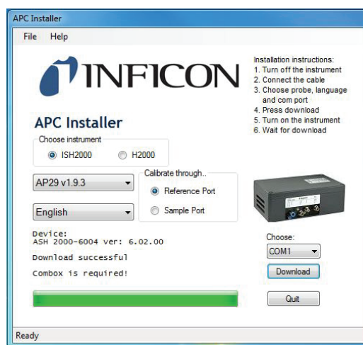
Figure F-5: APC Install after installation of software
