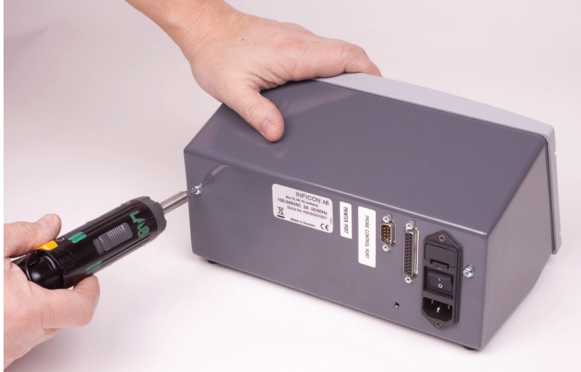
Figure E-7: Unscrew the two torx screws
