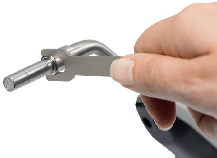
Figure E-25: Loosen the safety nut
