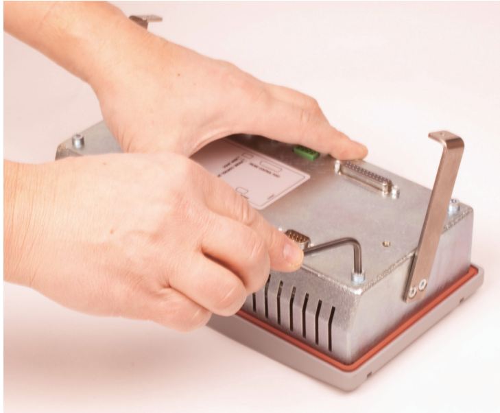
Figure E-15: Unscrew the two Allen Key Screws
