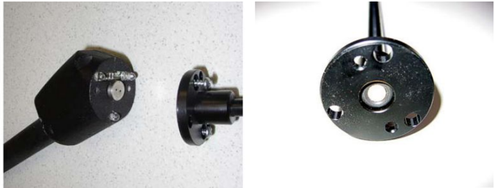
Fig. 18: Sinter filter in the sniffer handle
