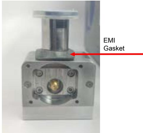
7. Remove the adhesive tape on the back of the new EMI gasket. Stretch the EMI gasket around the flange of the new MSC, with the adhesive side down and the cutout facing the spectrometer side. The cut out on the EMI gasket should align with the screw on the flange.
