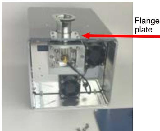
12. Stick the adhesive EMI gasket to the flange plate and the enclosure surrounding the flange of the MSC.
