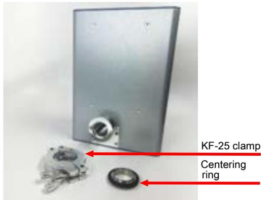
2. Attach the sensor cell flange on the system using the KF-25 centering ring and clamp.
